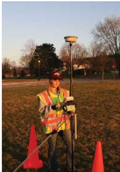
A surveyor with portable GPS, CORS, and up-to-date wireless can deliver accurate geospatial information in real time
