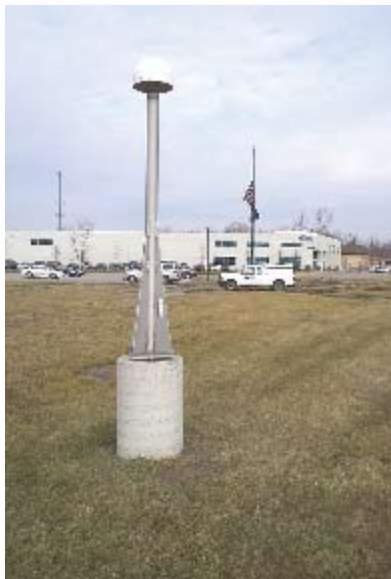
CORS stations such as this one are the backbone of the Michigan Spatial Reference Network (MSRN)
