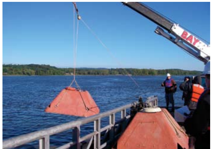
Figure 4. Deploying a current meter in Penobscot Bay, ME, from the US Coast Guard Cutter Abbie Burgess (above); and in the Hudson River, NY, from the Rosemary Miller , a contracted vessel (below).
