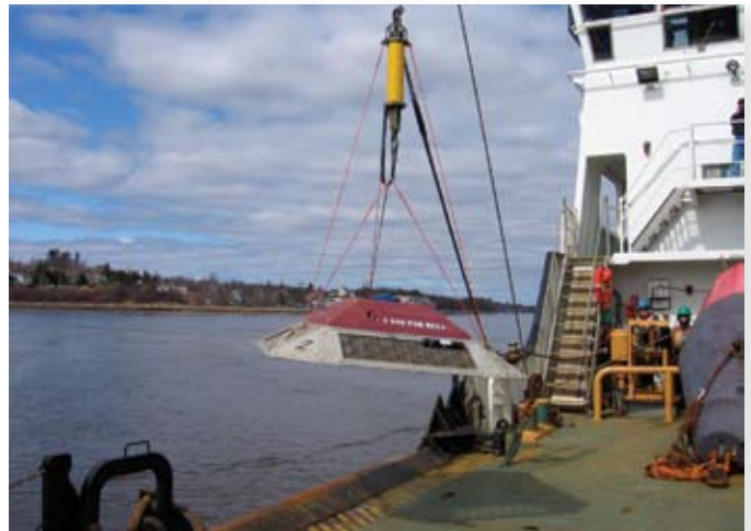
Figure 4. Deploying a current meter in Penobscot Bay, ME, from the US Coast Guard Cutter Abbie Burgess (above); and in the Hudson River, NY, from the Rosemary Miller , a contracted vessel (below).
