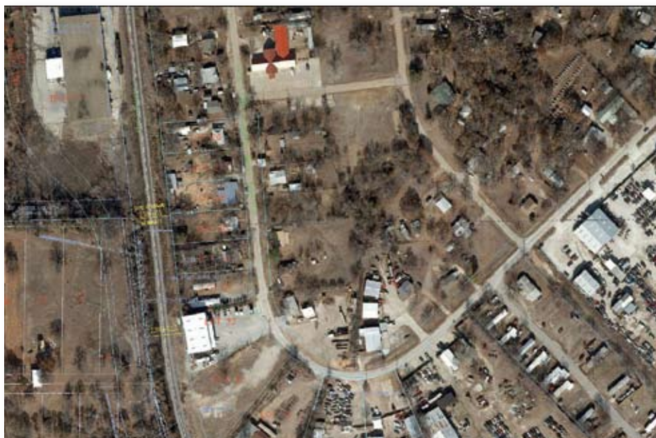
—An example of error when overlays, such as the orthophoto in this image, do not match the polygons of the parcel database
