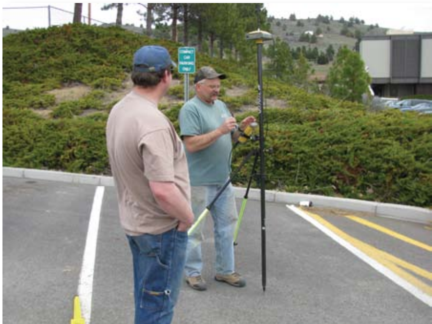
Students at Oregon Institute of Technology collect a point with a GPS receiver.
