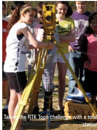
Measuring slope distance and angles to calculate elevation
