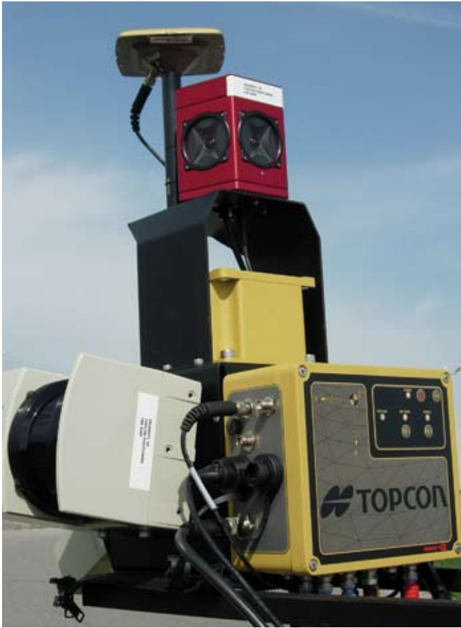
Topcon's IP-S2 uses high-accuracy GPS, an inertial measurement unit, 360-degree digital imaging, and a laser scanner to collect data for geospatial information systems.
